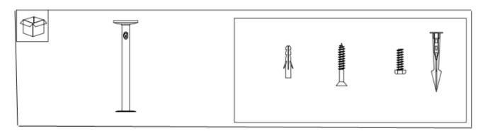
2. Install the fitting on the ground by locking the fitting base with screws and anchors.
