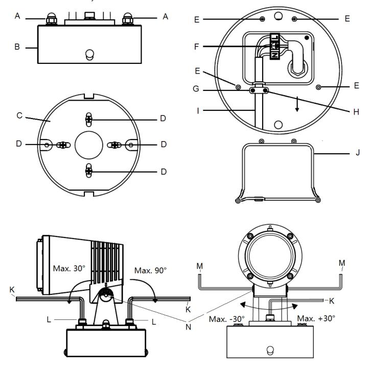
NOTE: When adjusting the head of the fitting, do not adjust more than angles shown in the above diagrams, as this may damage the wiring.
