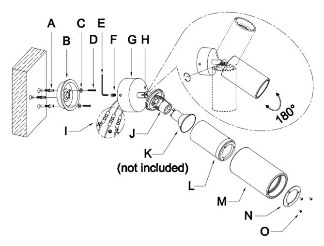
NOTE: DO NOT tilt the head up or down more than 180°. As this may damage the knuckle joint and the internal wires
