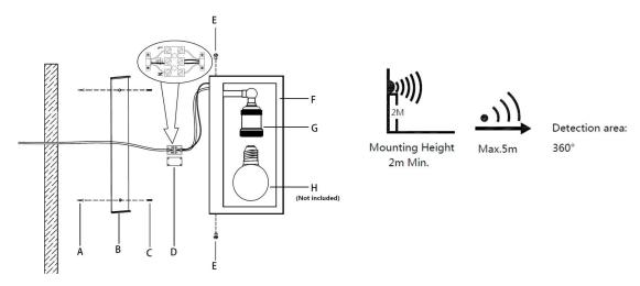
NOTE: MV sensor is sensitive to any moving objects. Vibration of the filament in the carbon filament lamps might also trigger the MV sensor. The light will switch off once the filament become static.
