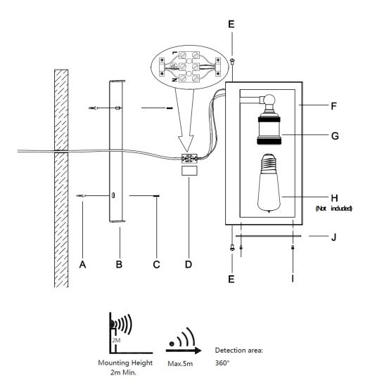
NOTE: MV sensor is sensitive to any moving objects. Vibration of the filament in the carbon filament lamps might also trigger the MV sensor. The light will switch off once the filament become static.
