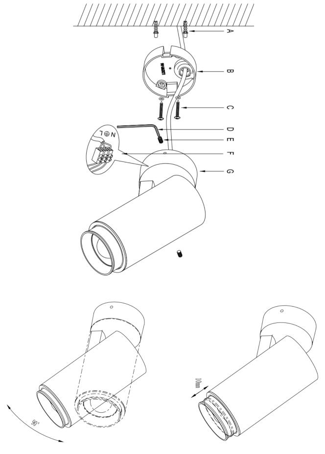
NOTE: Do not rotate/twist the shade more than 90°, as this may damage the joint or the internal wiring. NOTE: Do not adjust the outer shade more than 10mm, as this may damage the joint or the internal wiring.
