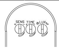
**SENS:** The detection distance of the sensor can be adjusted.
