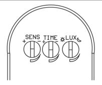
**<u>SENS</u>**: The detection distance of the sensor can be adjusted.
