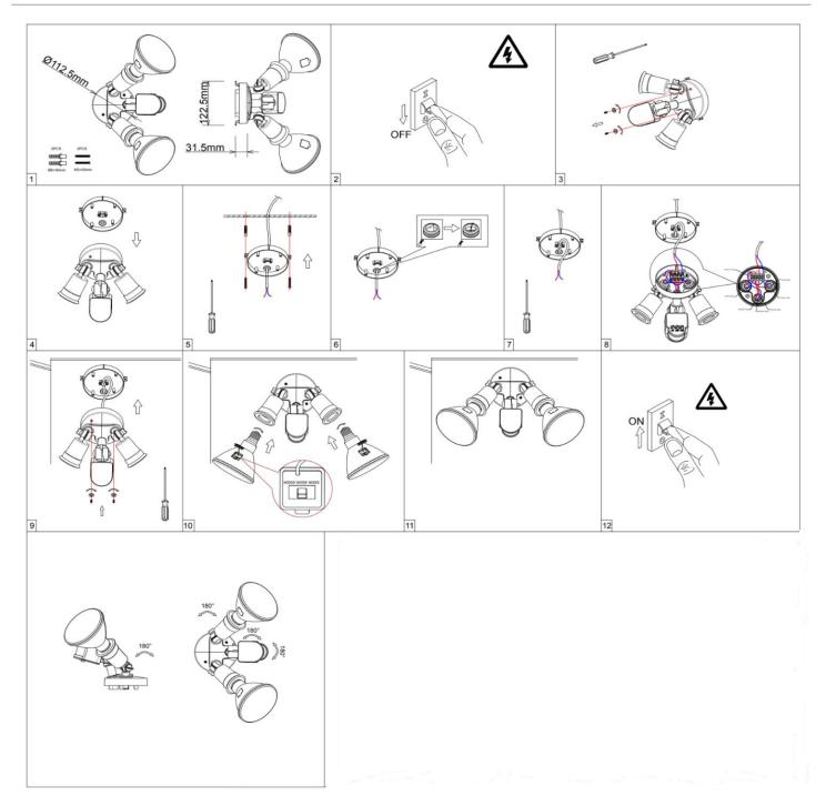
NOTE: Do not adjust the luminaire head more than 180° up and down, as this may damage the knuckle joint or the internal wiring.
