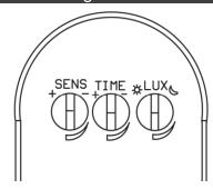
**SENS:** The detection distance of the sensor can be adjusted.
