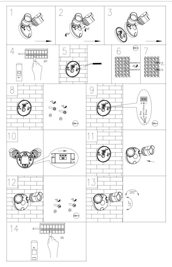
NOTE: Do not adjust the head more than 40° up and down, as this may damage the knuckle joint or the internal wiring.
