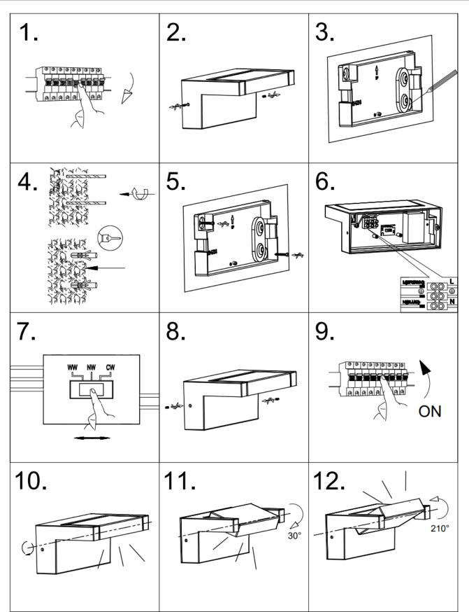
NOTE: Do not adjust the luminaire and up more than 210° and down more than 30°, as this may damage the internal wiring.
