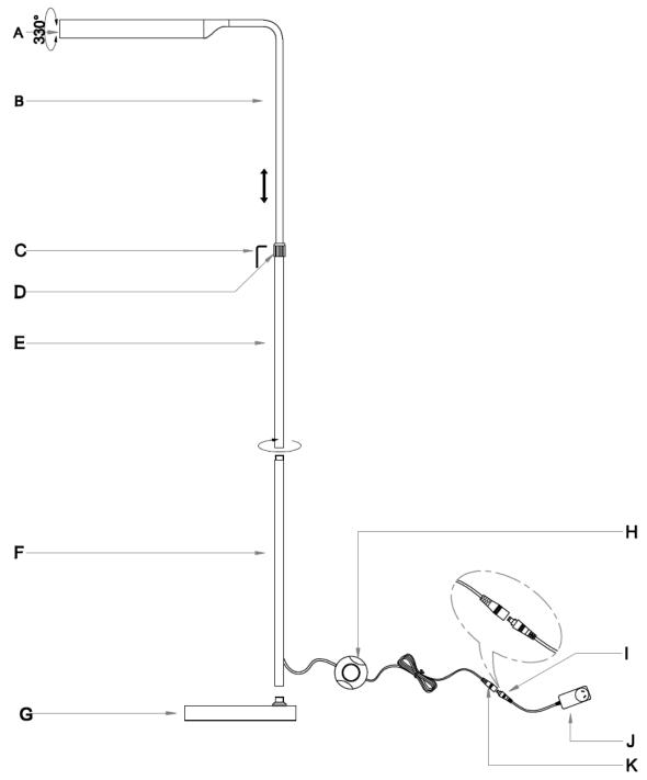
NOTE: Do not rotate the luminaire head (A) more than the 330° as this may damage the joint and internal wires.
