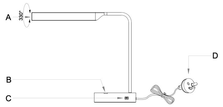
NOTE: Do not rotate the luminaire head (A) more than 330° as this may damage the joint and the internal wires.
