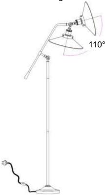
NOTE: When adjusting the arm of the fitting, do not adjust more than 110°. Refer to the picture below. Doing so may damage the internal wires and locking nut.
