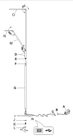
NOTE: When adjusting the pole (M), do not adjust more than 180° as this may damage the internal wires.
