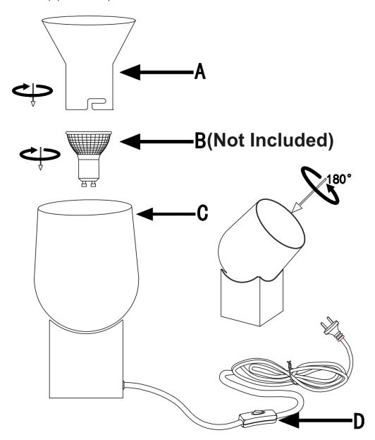
NOTE: Do not adjust the luminaire (C) more than 180°, as this may damage the joint or the internal wiring.
