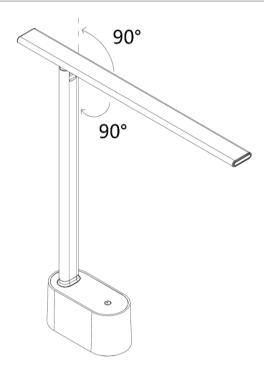
NOTE: Do not adjust the luminaire head up or down more than 90°, as this may damage the joint and the internal wires.
