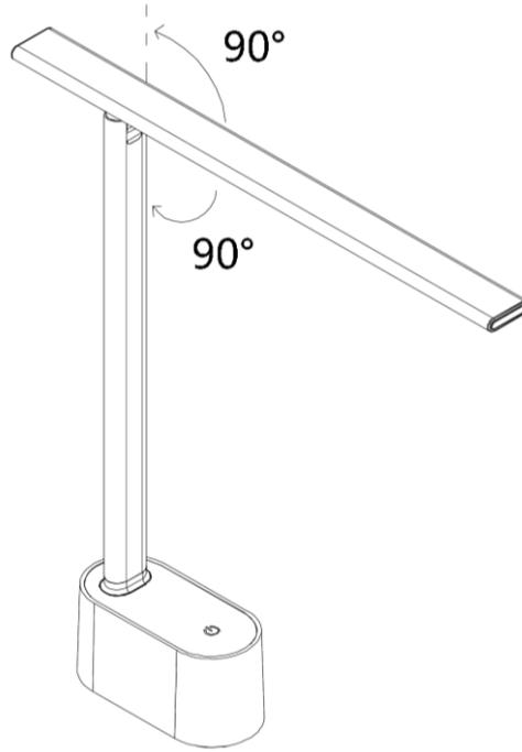
**NOTE: Do not adjust the luminaire head up or down more than 90°, as this may damage the joint and the internal wires.**
