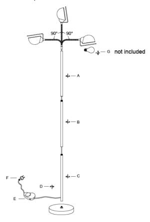
NOTE: When adjusting the head of the fitting, do not adjust more than 90°shown, as this may damage the wiring.
