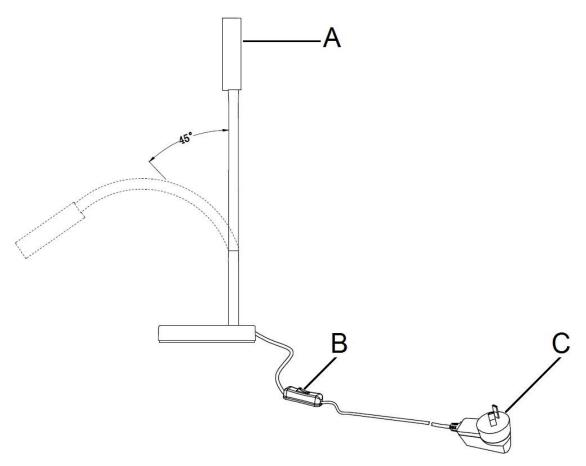
NOTE: When adjusting the head of the luminaire, do not adjust more than the 45° angle shown above, as this may damage the adjustable joint and the internal wires.
