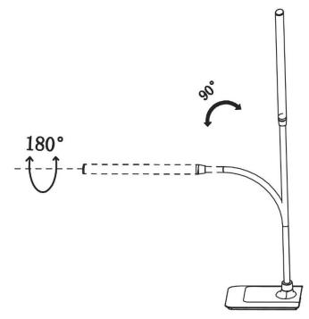
**NOTE:** When adjusting the angle of the head (B), do not rotate more than 180° as this may damage the internal wires. When adjusting the height of the head (B), do not adjust more than 90° as this may damage the internal wires.
