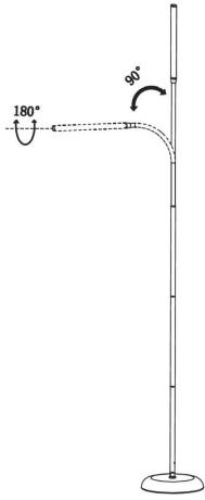
**NOTE:** When adjusting the angle of the head (B), do not rotate more than 180° as this may damage the internal wires. When adjusting the height of the head (B), do not adjust more than 90° as this may damage the internal wires.
