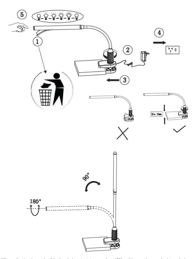
**NOTE:** When adjusting the angle of the head, do not rotate more than 180° as this may damage the internal wi res. When adjusting the height of the head, do not adjust more than 90° as this may damage the internal wires.
