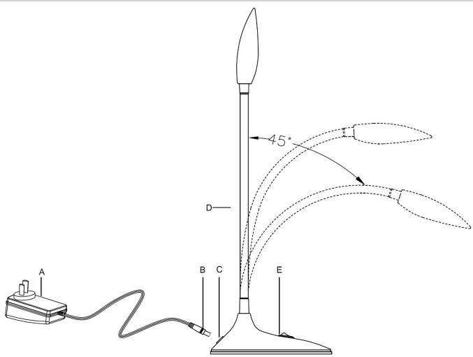
NOTE: When adjusting the angle of the arm (D), do not bend more than 45° as this may damage the internal wires.
