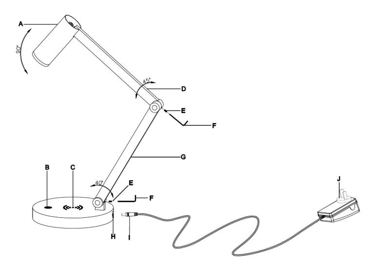
**NOTE:** When adjusting the head of the lamp (A), do not bend more than 90° as this may damage the internal wires.
