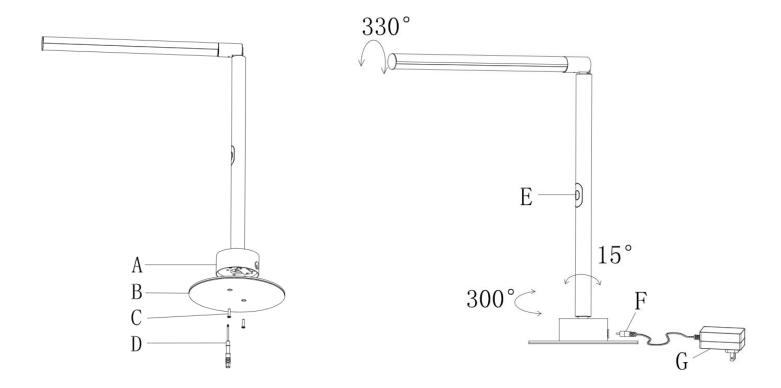
NOTE: When adjusting the head, do not rotate more than 330° as this may damage the internal wires. When adjusting the body, do not bend more than 15° as this may damage the internal wires. When adjusting the body, do not rotate more than 300° as this may damage the internal wires.
