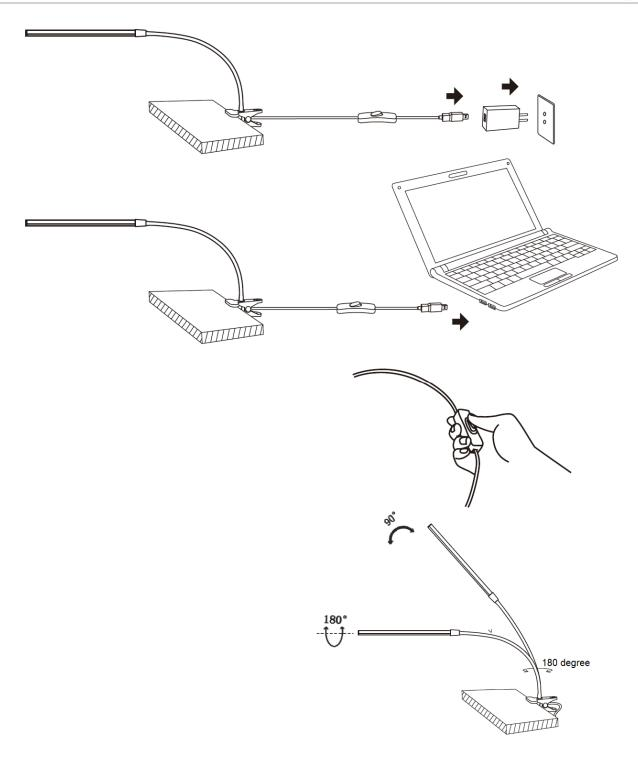
**NOTE:** When adjusting the angle of the head, do not rotate more than 180° as this may damage the internal wires. When adjusting the height of the head, do not adjust more than 90° as this may damage the internal wires.
