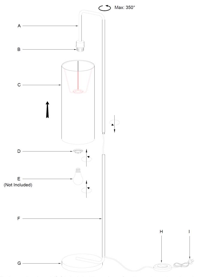
NOTE: Do not adjust the top half of the luminaire (A) more than 350°, as this may damage the socket and internal wires.
