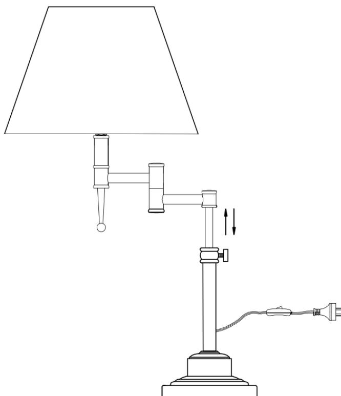
**ASSEMBLY DIAGRAM – Showing SKU# 260898 with Height adjustment**
