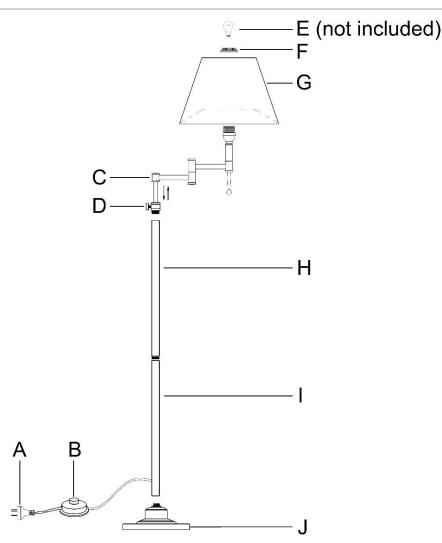
NOTE: The locking screw (D) must always be loosened before adjusting the telescopic arm (C) as this may damage the telescopic arm.
