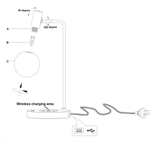
NOTE: DO NOT adjust lamp head over 90° vertically & 350° horizontally as this may damage the internal wires.
