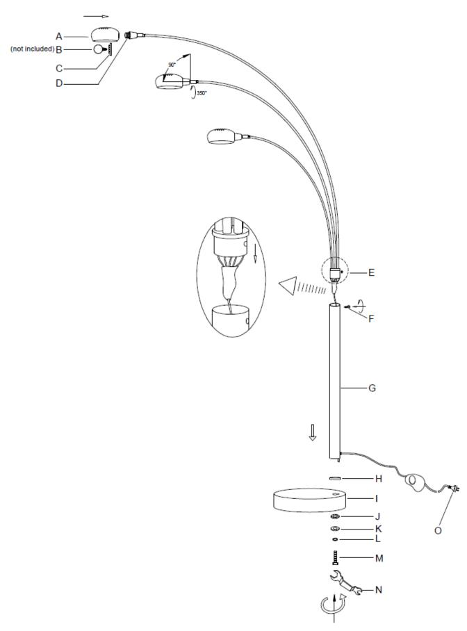
NOTE: Do not adjust the head up and down more than 90° and do not rotate the head more than 350° as this may damage the knuckle joint or damage the internal wiring
