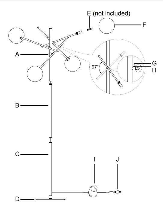
NOTE: Do not adjust the angle of the arm without first loosening the grub screw (H) with the allen key (G) provided, as this may damage the locking mechanism and will void warranty.
