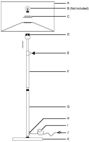
NOTE: The locking knob (E) must be loosened before adjust the height of the fitting.
