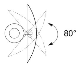
NOTE: Do not adjust the shade more than 80° as this may damage the knuckle joint.
