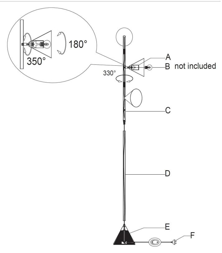
NOTE: Do not adjust the more than 180° and do not rotate the head more than 350° as this may damage the knuckle joint or damage the internal wiring.
