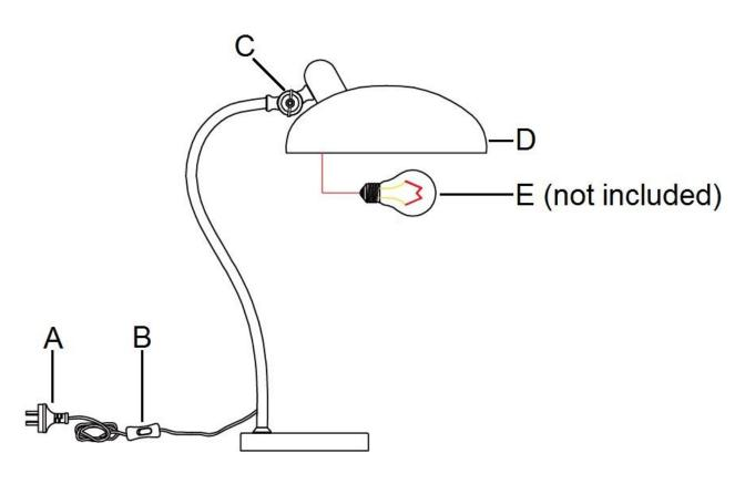
NOTE: When adjusting the shade (D), do not adjust more than 45° as this may damage the internal wires.
