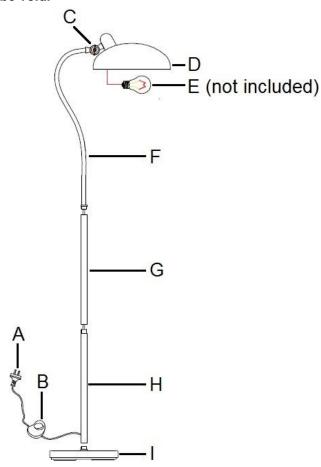
NOTE: When adjusting the shade (D), do not adjust more than 45° as this may damage the internal wires.
