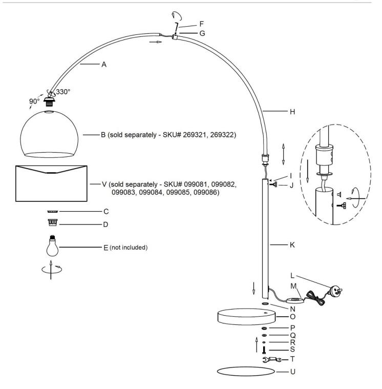
NOTE: Take care not to cross-thread or twist and damage the cord during assembly. Pull the cord out from the bottom section of the luminaire (K) as you assemble. Continuously check the cord during installation and relieve any twist in the cord by turning it in the opposite direction
