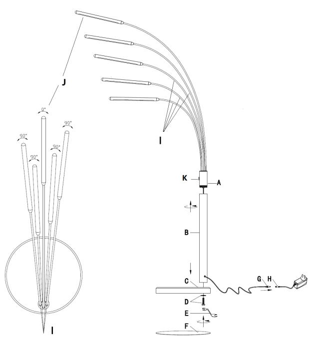
NOTE: When adjusting the LED head rods (I), do not adjust more than 90° as this may damage the internal wires.
