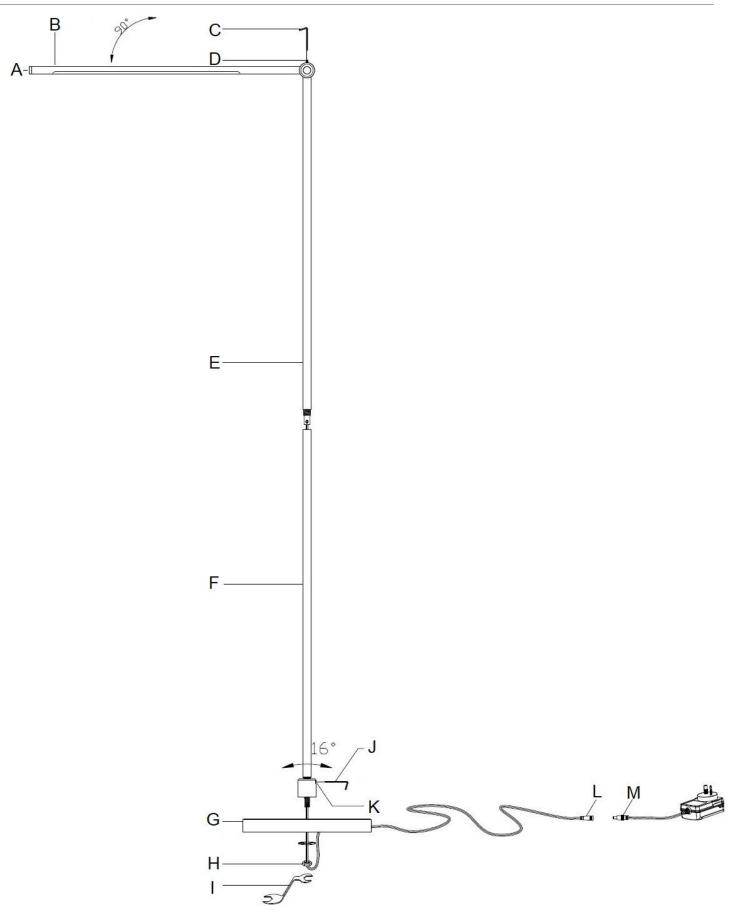
NOTE: Do not adjust the arm (B) more than 90°, as this may damage the knuckle joint or the internal wiring. NOTE: Do not adjust the body (F) more than 16°, as this may damage the knuckle joint or the internal wiring
