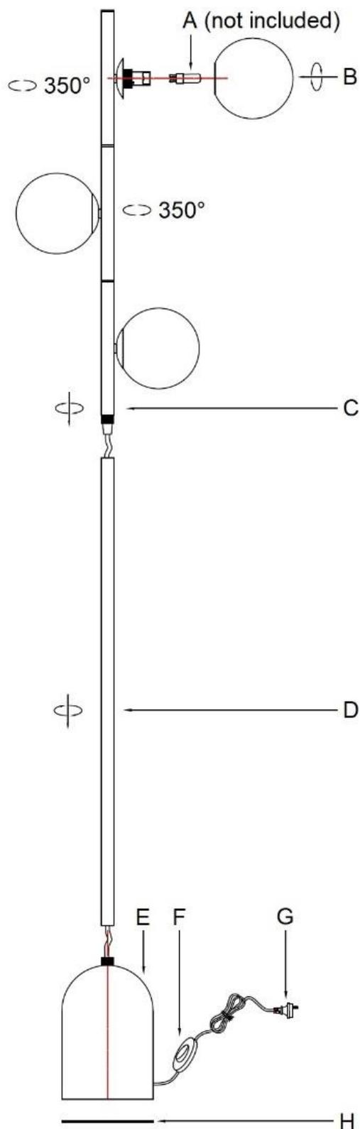
**NOTE: Do not rotate/twist the shade more than 350°, as this may damage the joint or the internal wiring.**
