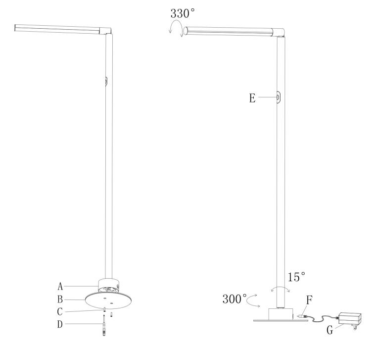
NOTE: When adjusting the head, do not rotate more than 330° as this may damage the internal wires. When adjusting the body, do not bend more than 15° as this may damage the internal wires. When adjusting the body, do not rotate more than 300° as this may damage the internal wires.
