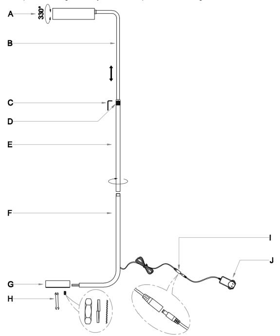
NOTE: Do not adjust luminaire head (A) more than the 330° as this may damage the joint and internal wires.
