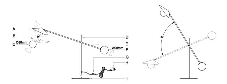
NOTE: Do not adjust the arm (E) more than 80°, as this may damage the joint or the internal wiring. NOTE: Do not adjust the head (A) more than 86°, as this may damage the joint or the internal wiring.
