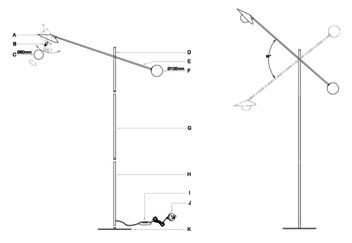
NOTE: Do not adjust the arm (E) more than 80°, as this may damage the joint or the internal wiring. NOTE: Do not adjust the head (A) more than 86°, as this may damage the joint or the internal wiring.
