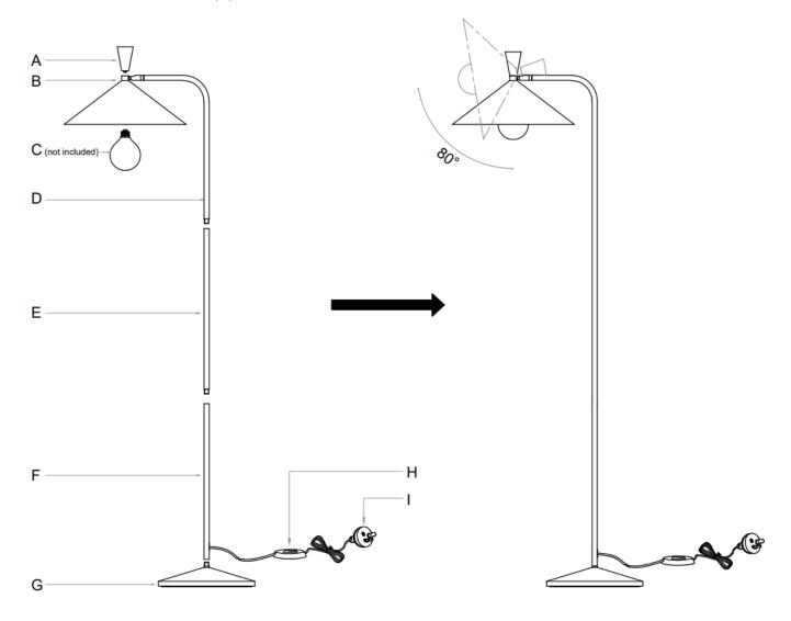
NOTE: Do not adjust the head more than 80° as this may damage the knuckle joint or damage the internal wiring.
