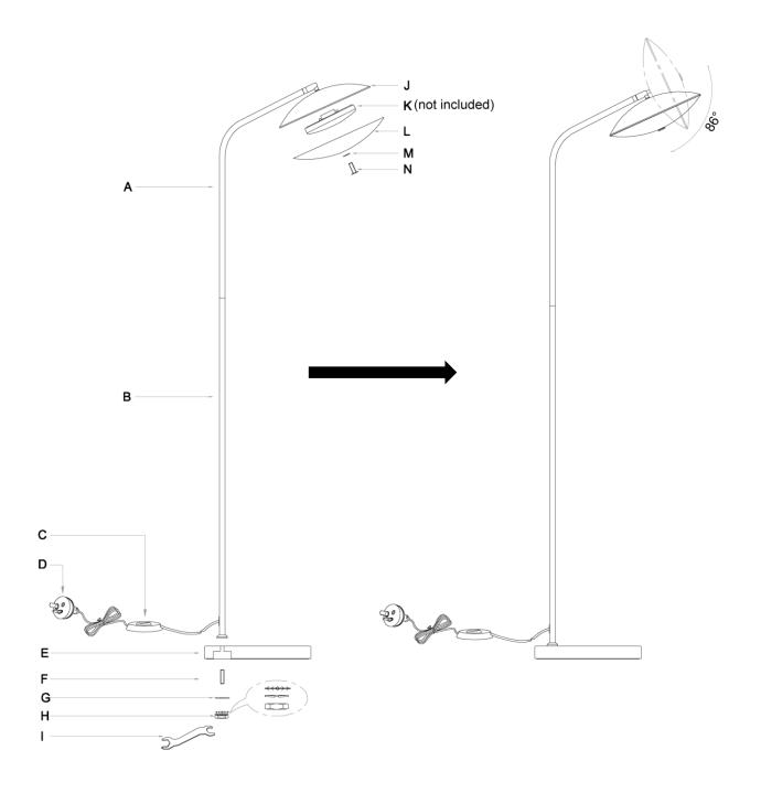
NOTE: Do not adjust the head more than 86° as this may damage the knuckle joint or damage the internal wiring.
