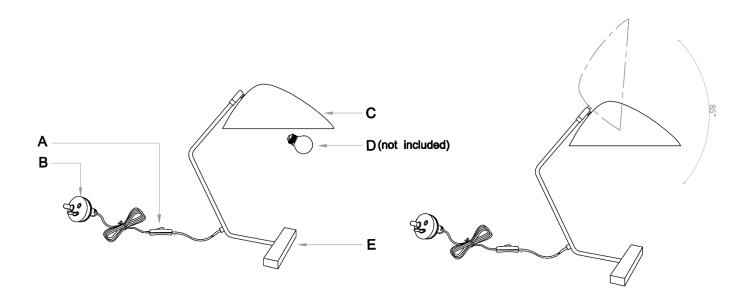
NOTE: Do not adjust the head more than 85° as this may damage the knuckle joint or damage the internal wiring.
