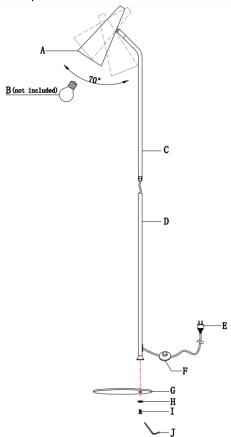
NOTE: Do not force or adjust the shade (A) more than 70°, as this may damage the joint or the internal wiring.
